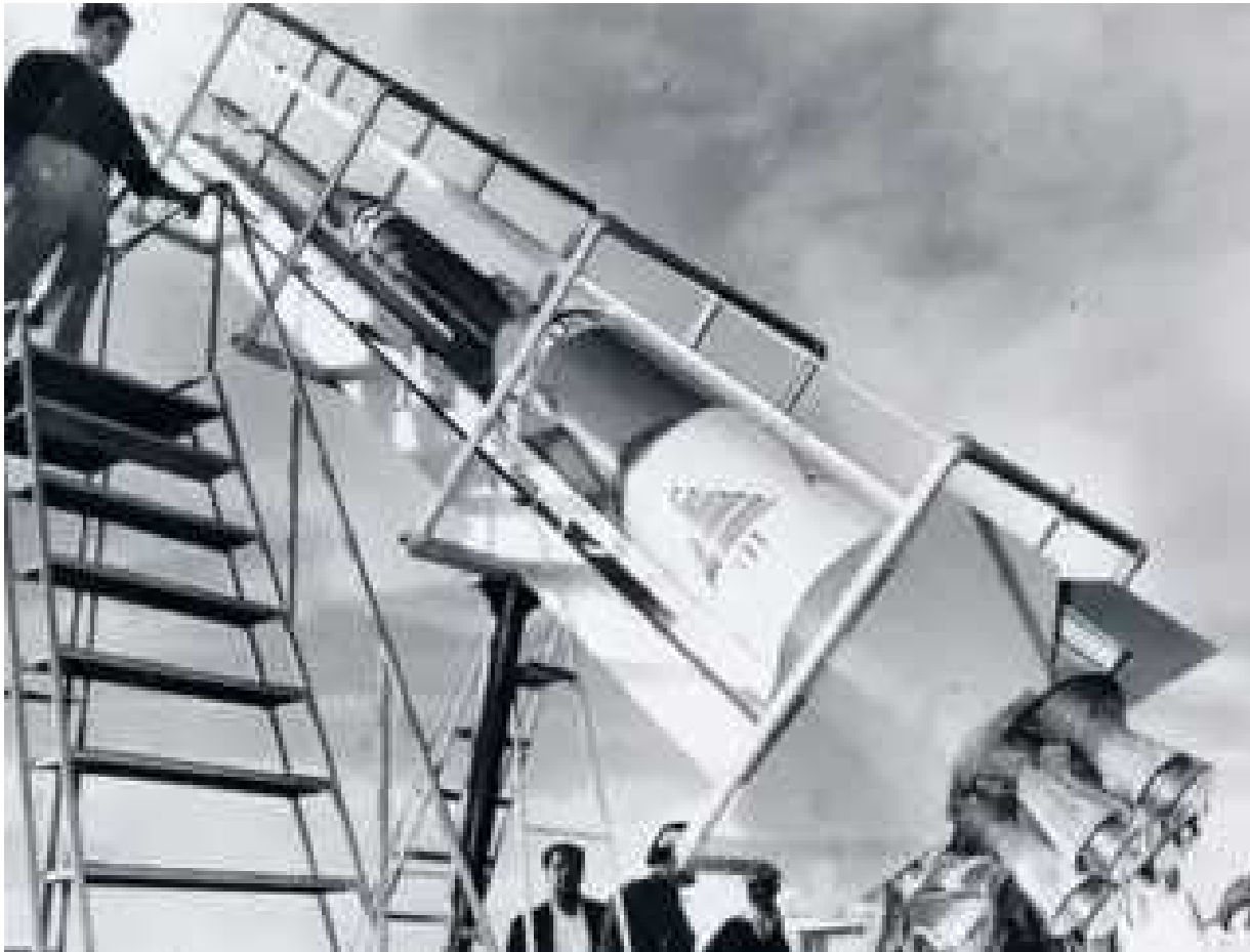
Cedar III launched in 1962 had a length of seven metres and weight of 1,250 kg
